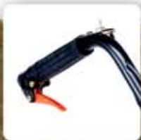
Right control incorporates throttle control and stop switch
